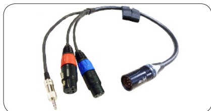
M3 MIXER END, 2' (2) XLR 3-PIN TO XLR 7-PIN MALE
